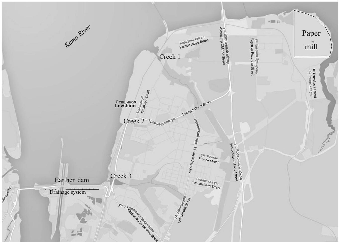
Fig. 1. Potential sources of organic substance inflow into a dam embankment.
